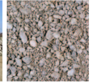
Recycled concrete aggregate
