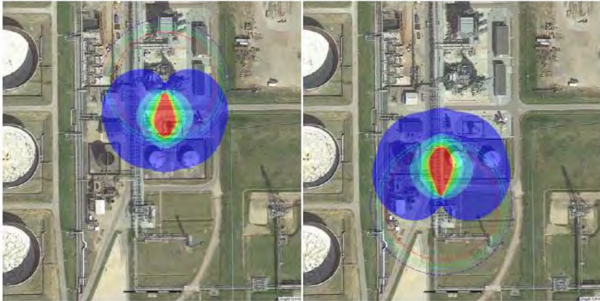
Figure 6-1 Copy of Figur IV-101 Heat radiation from a jet fire with a large release (120 mm) from a loss of containment at V-9625 or V-9903 with contours for 5 kW/m 2 (blue), 9,4 kW/m 2 (turquoise), 15 kW/m 2 (green) and 35 kW/m 2 (red)
