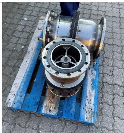
Afmonteret break away kobling
