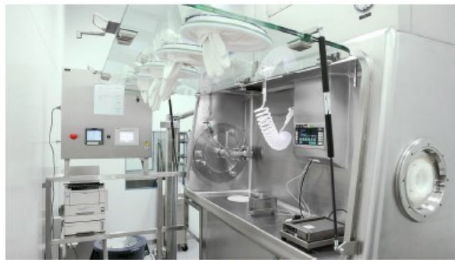
Figur 8: Isolator example B
