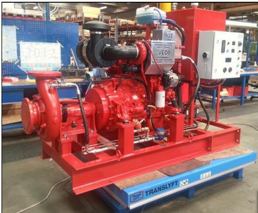
Foto 2 – Dieseldrevet brandvandspumpe DESMI/Caprari
