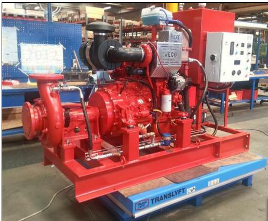
Foto 2 – Dieseldrevet brandvandspumpe DESMI/Caprari
